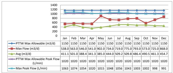
The above table shows there were spikes in <u>instantaneous</u> peak flow rate (L/min) and max flow rate these occurrences were caused during pump start-up/pump to waste. The Peak Flow rate was increased in May 2021 during scheduled flow meter calibrations.
