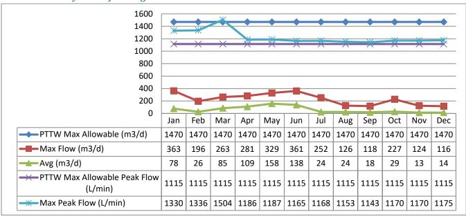
The above table shows there were spikes in <u>instantaneous</u> peak flow rate (L/min) and max flow rate these occurrences were caused during pump start-up/pump to waste. The Peak Flow rate was increased in May 2021 during scheduled flow meter calibrations.
